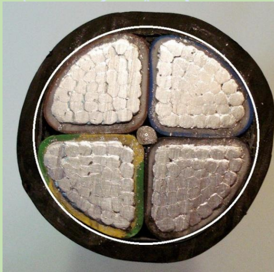
Photo 8. Compaction & roundness are very well.
