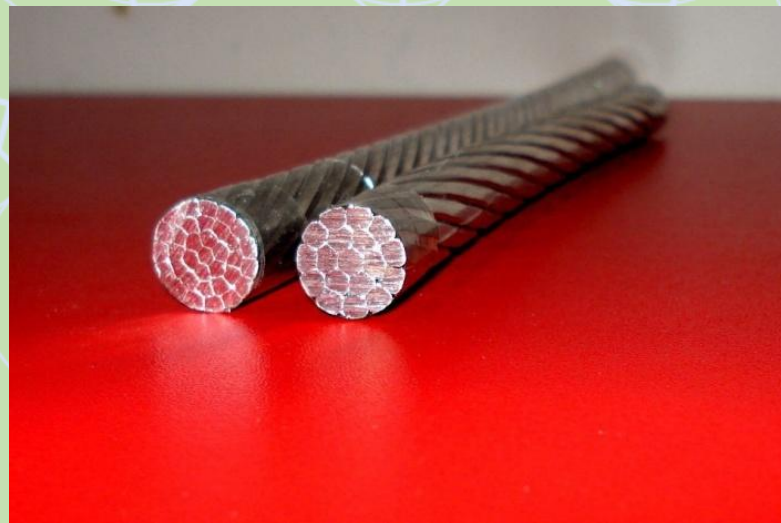
Photo 4. The same cross section, but are with different arrangement and diameter of wires.
