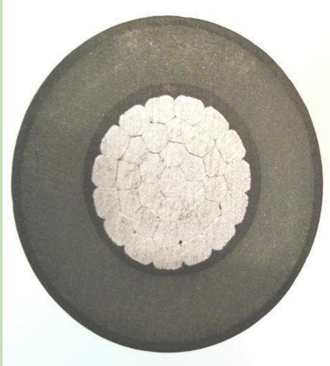
Photo 2. This conductor is compacted with rollers.
