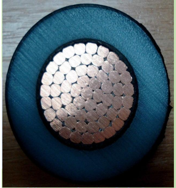
Photo 3. This conductor is compacted with hard dies
