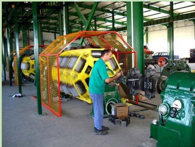
Photo 12. This is very old rigid stranding machine.
