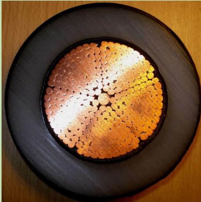
Photo 10. Milliken conductor with segments manufactured with using horizontal rollers.
