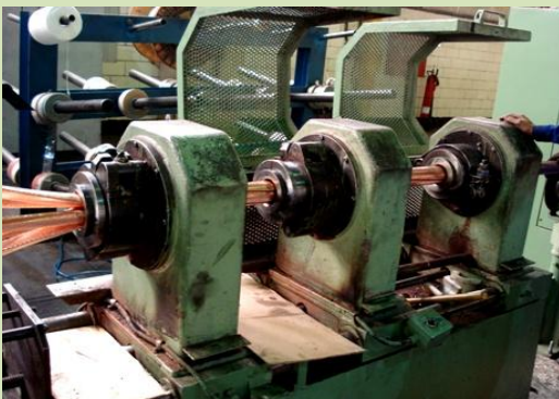
These assembly dies are manufactured in MIROSCABLE ENGINEERING Company and delivered to RCGC.
