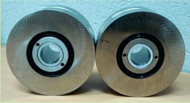
The complete assembled pair of rollers for round form
