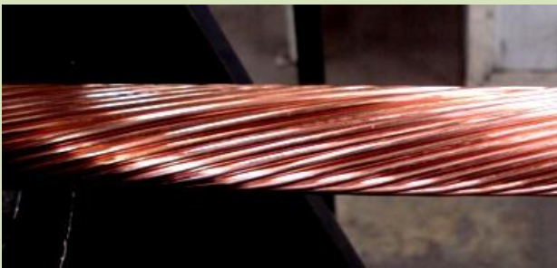
The problem of uneven tension of wires is solved with specially molded dies for the sector and round compacted conductors.
