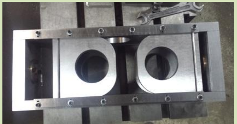
Connecting multiple cassettes in a block for compaction is very simple.
