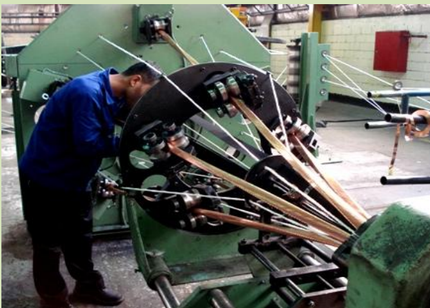
We have an original design and produce a set of dies for assembly stranding sector shaped conductors for Milliken cables.
