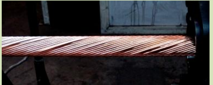
The problem of uneven tension of wires is solved with specially molded dies for the sector and round compacted conductors.
