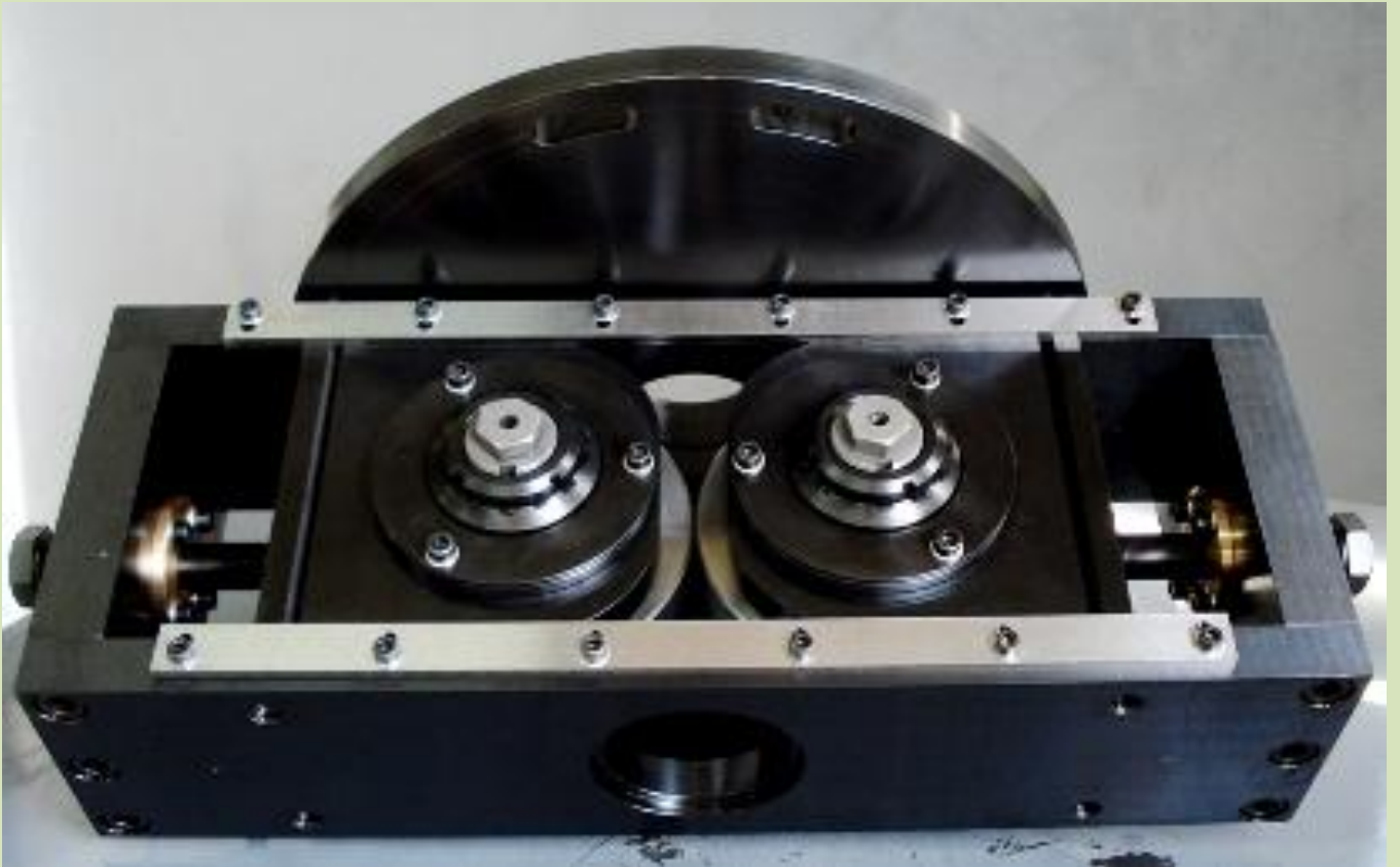
The Centering and parallelism of the rollers is always correct.
