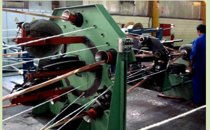
We have an original design and produce a set of dies for assembly stranding sector shaped conductors for Milliken cables.
