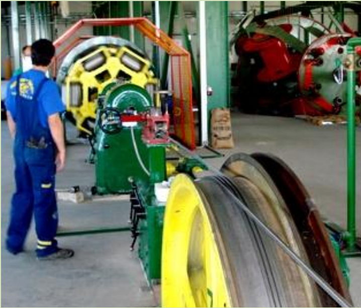
The capstan with one wheel has enough pulling power for compacting with rollers.
