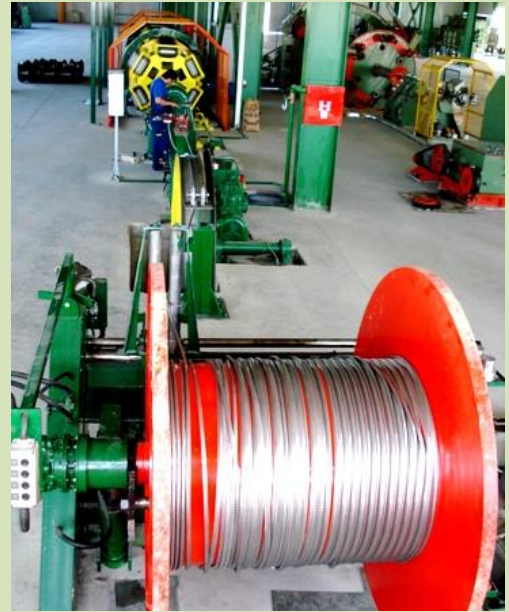
The capstan with one wheel has enough pulling power for compacting with rollers.
