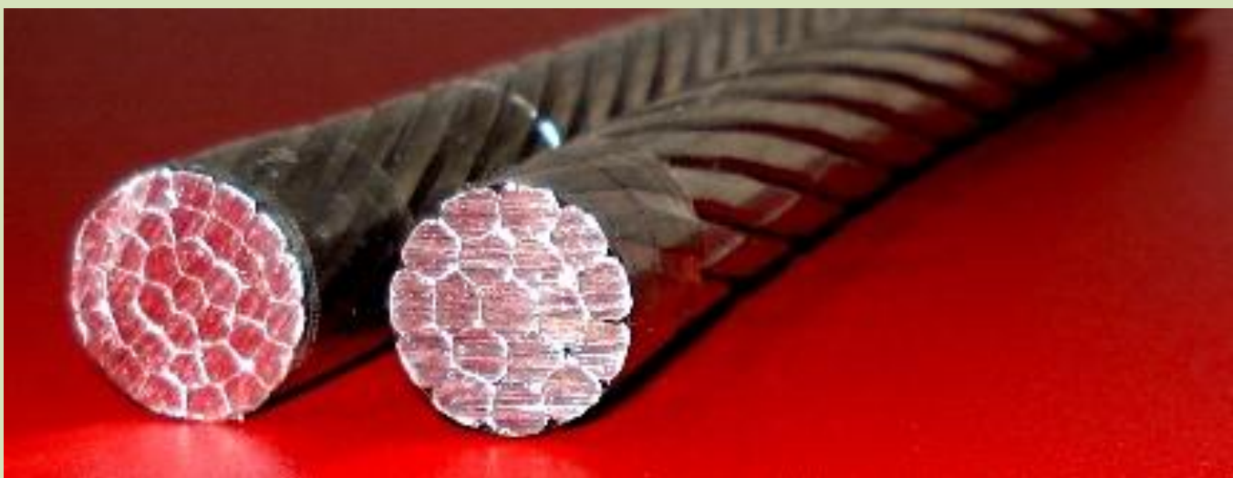
The same conductor cross-section but it is a different number and diameter of the wires.
