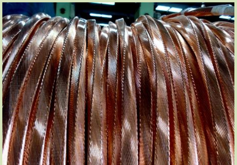
The sector shaped conductor is really excellent.
