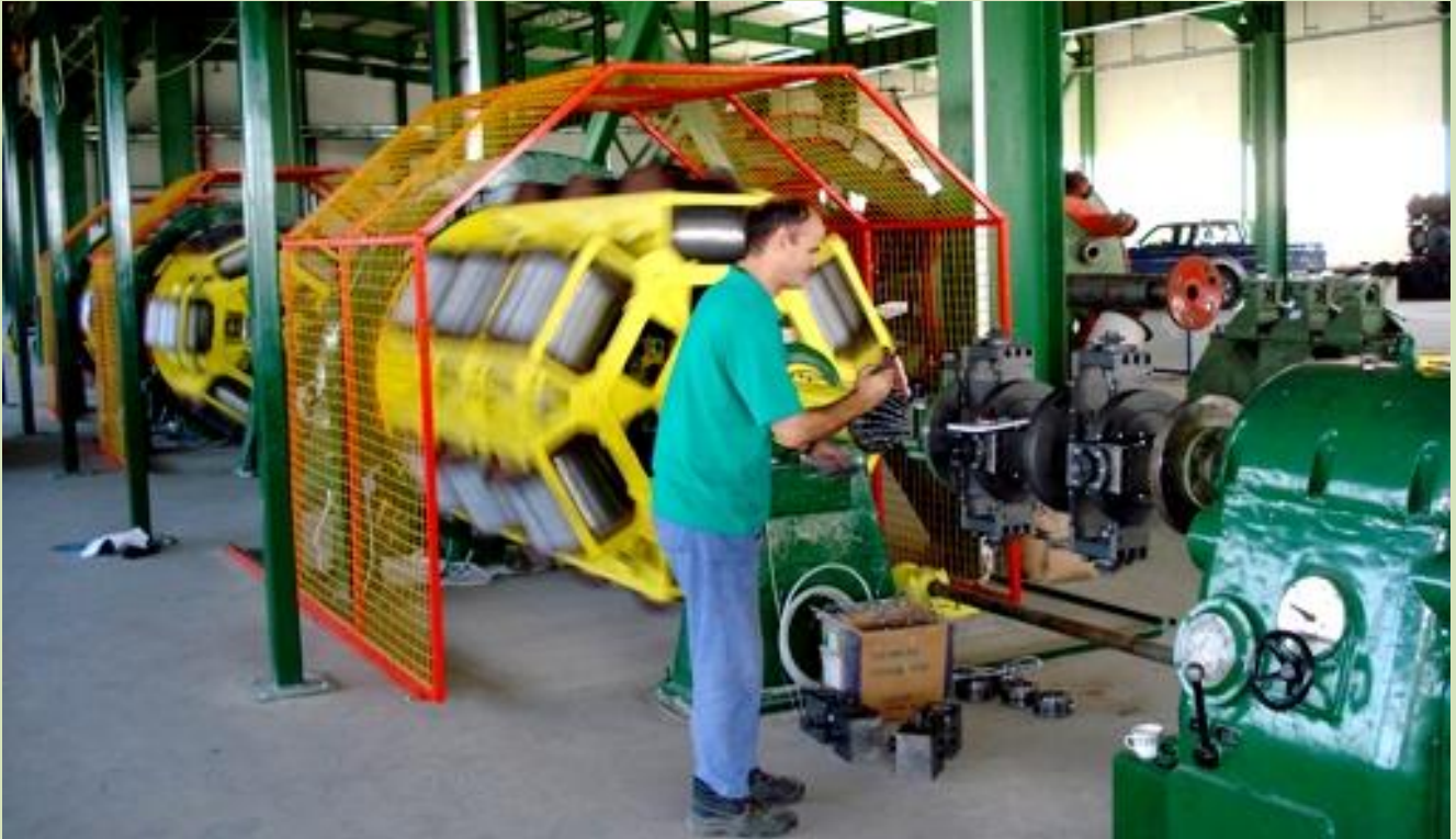
This stranding line is old about 100 years, but with new design rollers and new cassettes produces exelent compacted conductors.
